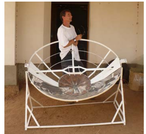
Roberto with his partially finished parabolic cooker.
